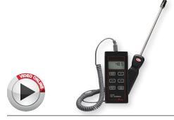
The **Model 485B Thermo-Hygrometer** is a versatile, compact, handheld instrument for measuring percentage of relative humidity and temperature in °F or °C. Dew point and wet bulb temperatures are derived from the relative humidity and temperature measurements and are displayed on the LCD.
