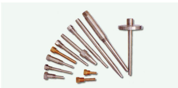
SHTR-17 Thermowell for thermocouple and RTD IEC standard, protection tube with one piece material machined, no welding, maximal deep blind hole up to 1.5m, bearing high temperature and high pressure, corrosion-resistant type and flanged type available.
